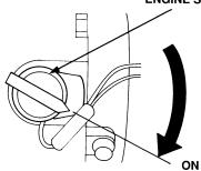
Figure 12. Engine ON/OFF Switch (ON Position)
